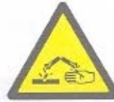
Caution, corrosive substance
